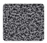
Cellulose nitrate membrane filters are indicated for many general laboratory applications where a membrane with a high non-specific adsorption is suitable. They are hydrophilic, have high flow rates thanks to their symmetric structure and are compatible with aqueous solutions (pH 4-8),
