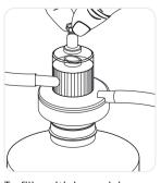
To fill multiple receiving bottles, break the vacuum with the valve on top of the Sartolab® 150v housing.
