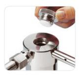
A practical filter holder for many laboratory filtrations. It can be attached to a tripod with the help of a steel rod which can be screwed in. The hose nipple is screwed into the side of the top part, leaving room for a large filling opening. This makes pouring in the sample easier, and the sample can be refilled without removing the tube connection to the pressure source. Leak-proof sealing is achieved by hand-tightening the
