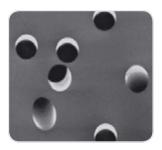
Those white and hydrophilic polycarbonate track-etched membranes are manufactured from high grade polycarbonate film using track-etch technology. Their capillary pore structure is uniform and precise, with a narrow pore size distribution to retain particles on their surface. Track-etched membranes are an excellent choice for accurate fractionation of particulates
