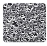
Polyethersulfone (PES) membrane filters are hydrophilic, have high flow rates thanks to their symmetric structure, have a low non-specific protein adsorption and are chemically resistant over a pH range of
